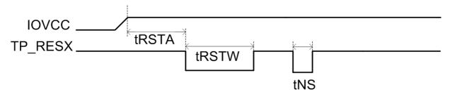
Conditions:  $IOVDD = 1.65V \sim 1.95V$ , GND = 0V,  $T_A = -20^{\circ}C \sim 85^{\circ}C$
