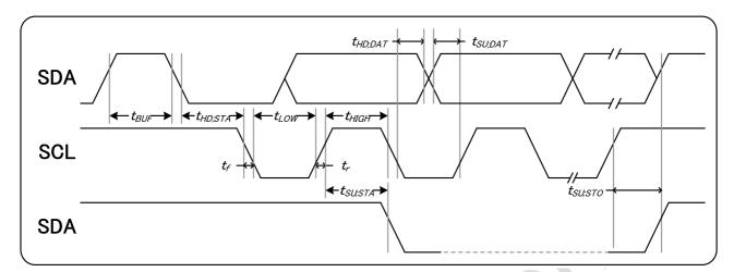
Conditions:  $IOVDD = 1.65V \sim 1.95V$ , GND = 0V,  $T_A = -20^{\circ}C \sim 85^{\circ}C$
