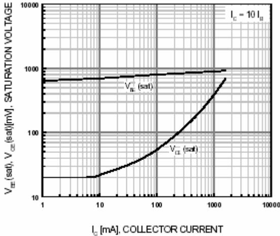
Figure 3. Base-Emitter Saturation Voltage
