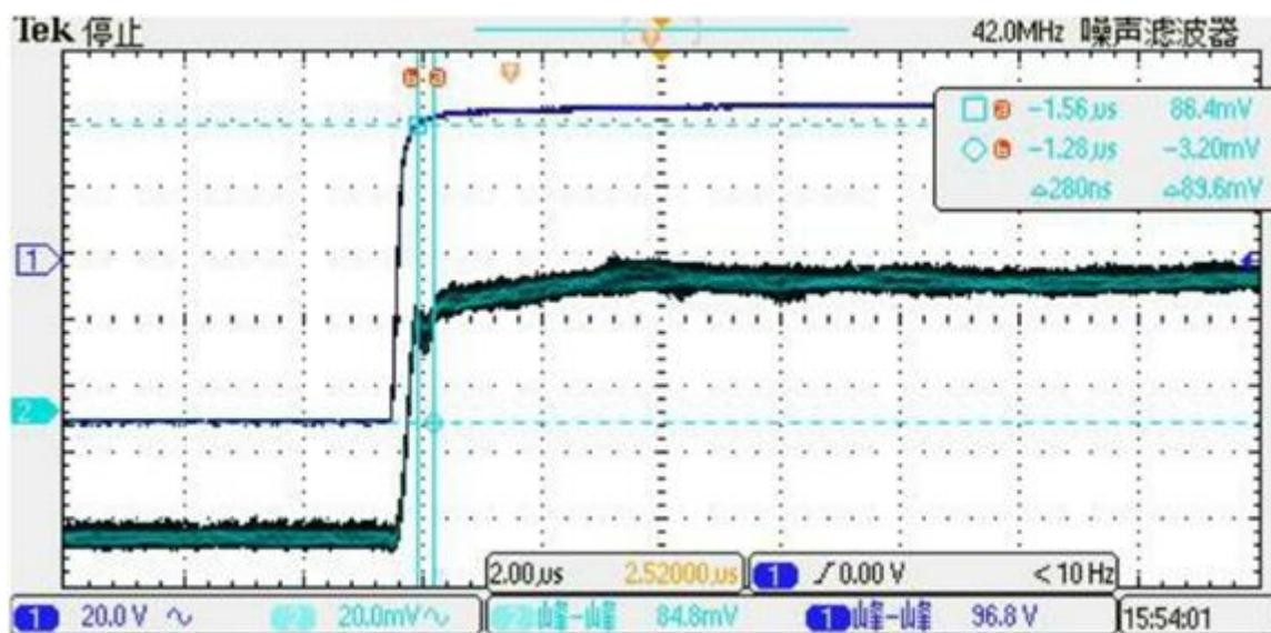
The step response time of STB-xxCAS/F current sensors. The blue is primary current, while the green is output signal of current sensor. The step response time is less than 0.3  $\mu$ s.
