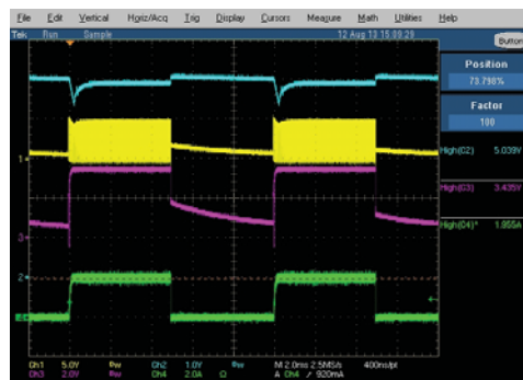
Figure 26. 100 Hz PWM dimming function
