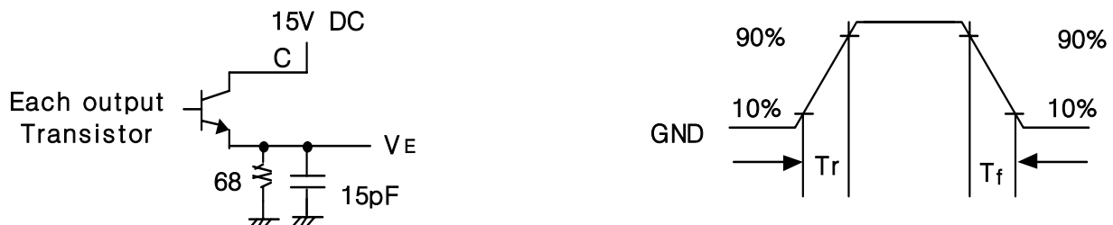
Fig. 4 Emitter-Follower Configuration Test circuit and waveform Voltage waveform
