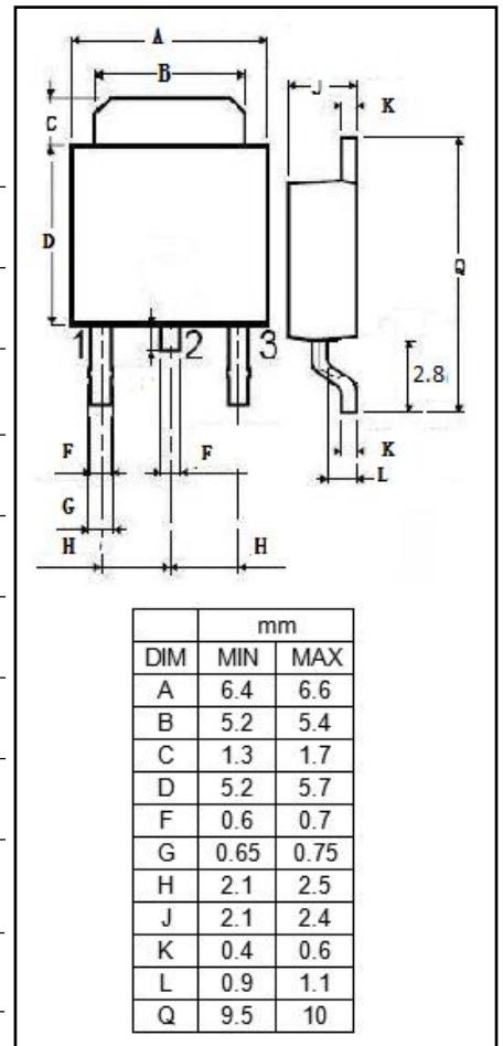
**isc N-Channel MOSFET Transistor****STD4NK60ZT4****ELECTRICAL CHARACTERISTICS****T<sub>c</sub>=25°C unless otherwise specified**
