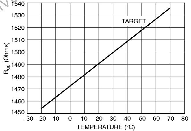
Figure 4. R<sub>UP</sub> versus Temperature
