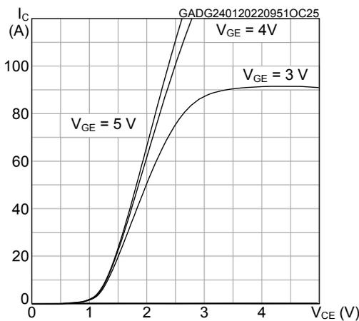
**Figure 4. Typical output characteristics (T<sub>J</sub> = 175 °C)**
