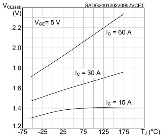
**Figure 6. Typical V<sub>CE(sat)</sub> vs collector current**
