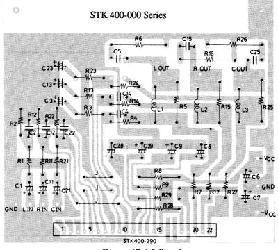
Copper (Cu) foil surface In the STK401-000 series, pin No. 6 corresponds to pin No. 1.
