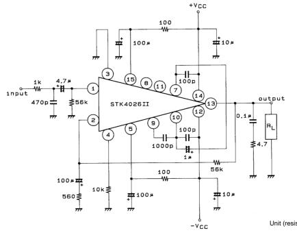
Unit (resistance:  $\Omega$ , capacitance: F)
