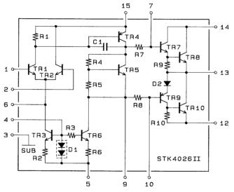
Sample Application Circuit: 25 W min AF Power Amplifier
