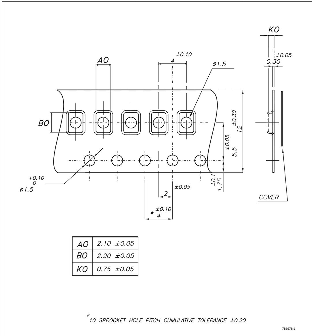
Figure 11. Reel information for QFN12 (2.2 x 1.5 x 0.5 mm) - 0.40 mm pitch
