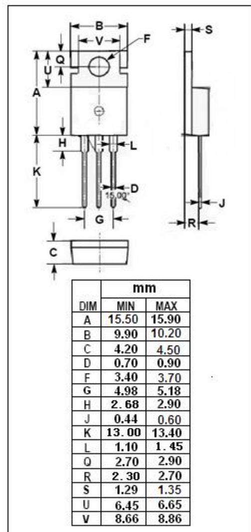
**Isc N-Channel MOSFET Transistor****STP16NF06****ELECTRICAL CHARACTERISTICS****T<sub>C</sub>=25°C unless otherwise specified**
