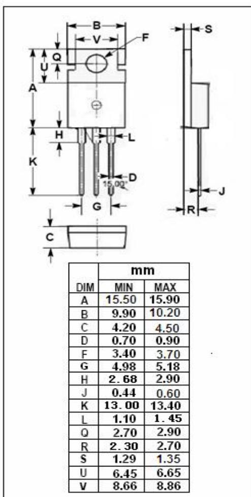
**Isc N-Channel MOSFET Transistor****STP30NF10****ELECTRICAL CHARACTERISTICS****T<sub>c</sub>=25°C unless otherwise specified**
