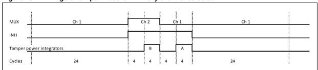
When the secondary channel is selected to be integrated by the final energy integrator, the MUX and INH signals change according to *Figure 19* below.
