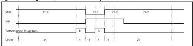
Figure 19. Timings of tamper module - Secondary channel selected
