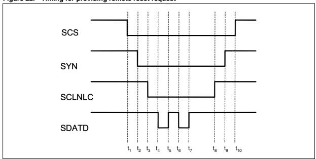
Figure 22. Timing for providing remote reset request (1)
