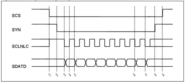
$t_1 \rightarrow t_2$  (> 30 ns): SPI out of idle state
