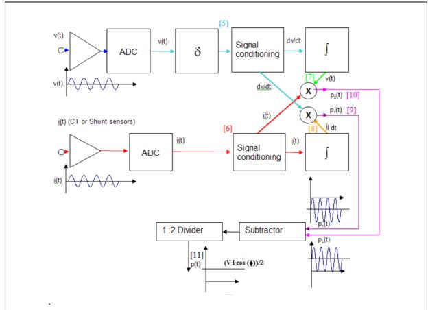
Figure 26. Active energy computation diagram
