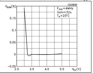
Figure 11. Error over dynamic range gain dependence
