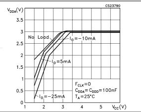
Figure 7. Digital voltage regulator: line - load Figure 8. regulation
