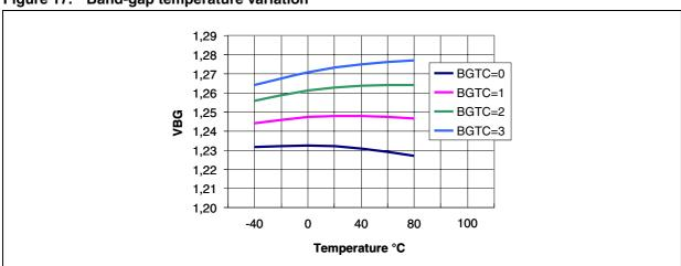
Figure 17. **Band-gap temperature variation**
