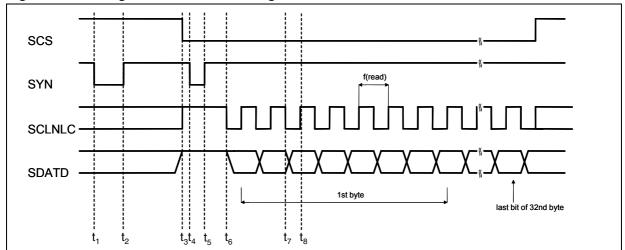
Figure 24. Timing for data record reading
