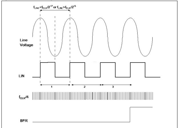
If the number of pulses counted between two trailing edges of LIN is lower than  $2^{13}$ , the base frequency exceeds the limit (this means it is higher than  $f_{CLK}/2^{15}$ ). In this case, the error must be repeated three consecutive times in order to set the BFR error flag.
