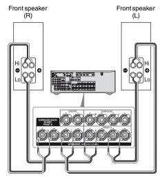
Connect the jacks on the Lo (or Hi) side of the front speakers to the SPEAKERS FRONT A terminals, and connect the jacks on the Hi (or Lo) side of the front speakers to the SPEAKERS SURROUND BACK/BI-AMP/FRONT B terminals.
