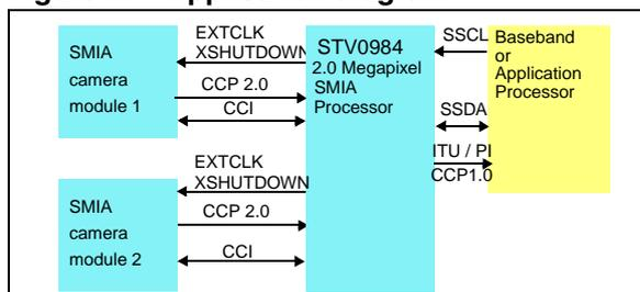
**Figure 2. Block Diagram**
