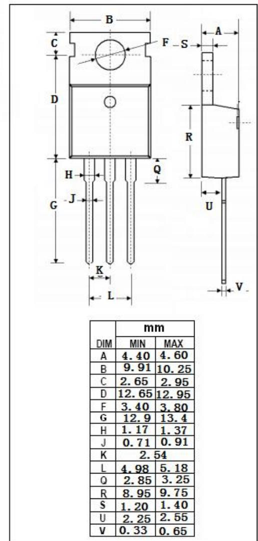
**Isc N-Channel MOSFET Transistor**
