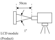
Luminance Meter (TOPCON BM-5A) Spectroradiometer (TOPCON SR-3)
