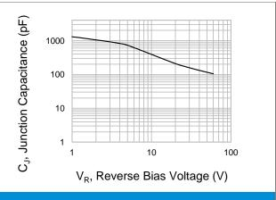
Fig.2 Typical Junction Capacitance
