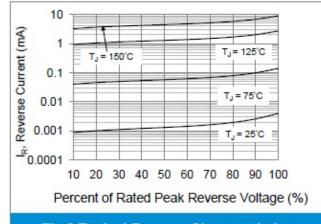
Fig.3 Typical Reverse Characteristics
