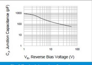
Fig.2 Typical Junction Capacitance
