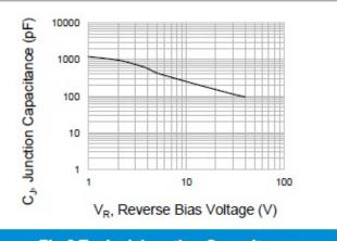
Fig.2 Typical Junction Capacitance
