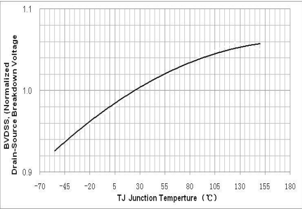
Fig 5. Breakdown Voltage Variation vs. Junction Temperature
