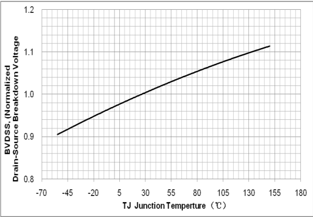
Fig 5. Breakdown Voltage Variation vs. Junction Temperature
