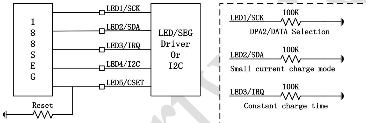
In discharge mode, segment will keep on to indicate battery capacity. When battery capacity is lower than 5%, segment will flicker with frequency of 1Hz. When battery is low power, segment 0% will flicker 5 times to indicate battery needs to charge and then power off.
