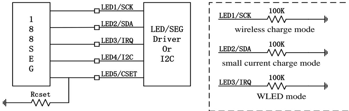
The fast charge 188 segment type is KHP302518, and is set when LED4/I2C pin connects a 100K  $\Omega$  resistor to ground. Its mechanical outline and circuit diagram is as below:
