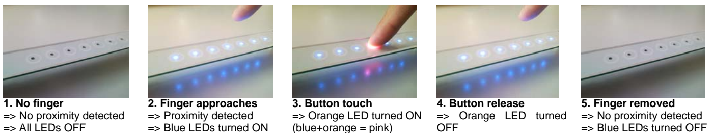
Figure 60 Touch+Proximity Module Operation
