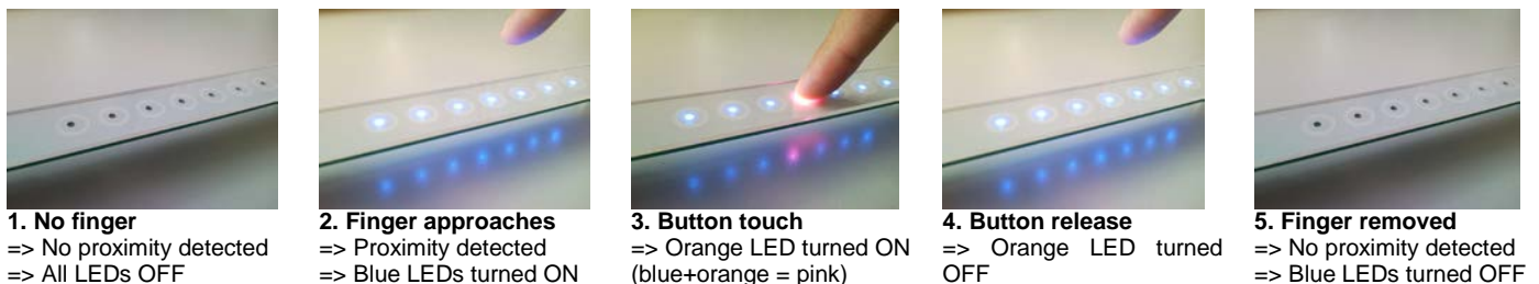
Figure 64 Touch+Proximity Module Operation
