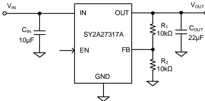
Figure 1. Schematic Diagram
