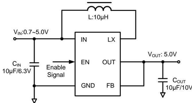
Figure 1. Schematic Diagram
