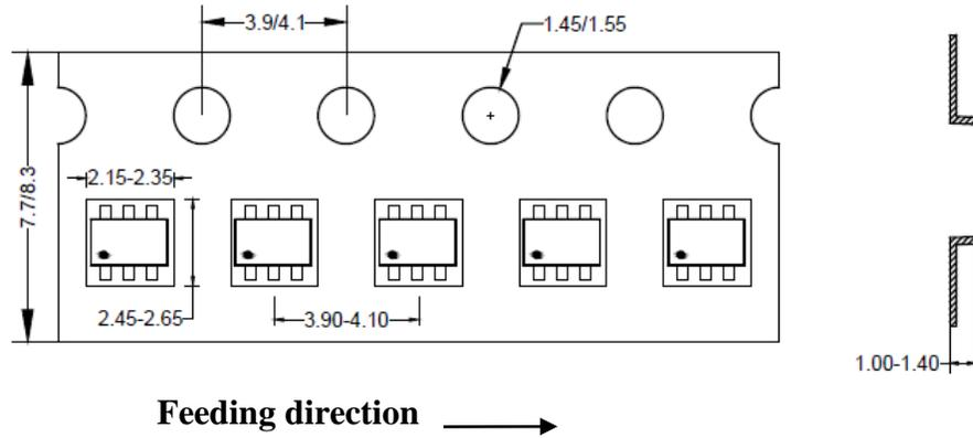
**2. Carrier Tape & Reel specification for packages**
