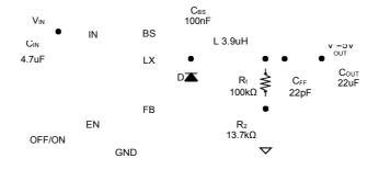
Figure 1. Schematic Diagram
