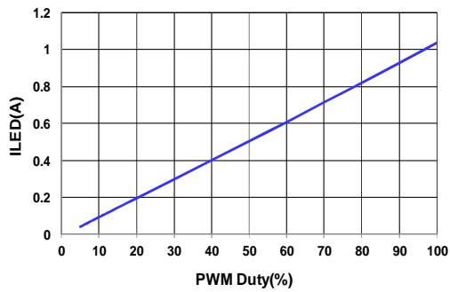
PWM Dimming: PWM Duty vs. LED Current (L=6.8uH, I o =1A, V in =15V, 3 pcs LED Series)
