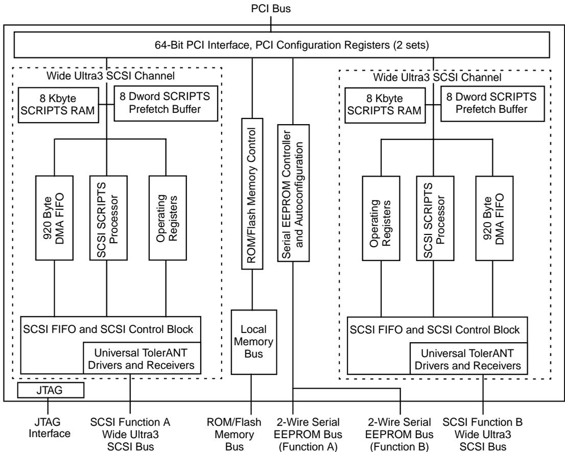
The SYM53C1010 has two wide Ultra3 SCSI channels in a single package. Each SCSI channel (A and B) incorporates an independent DMA FIFO and a separate internal 8 Kbyte SCRIPTS RAM.
