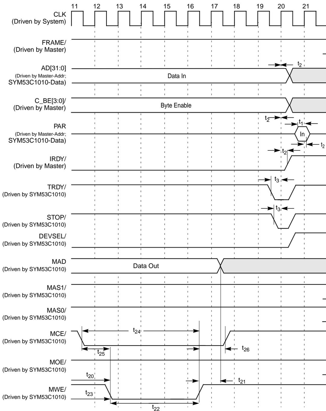
**Table 6.33 Normal/Fast Memory ( $\geq 128$  Kbytes) Single Byte Access Read Cycle**
