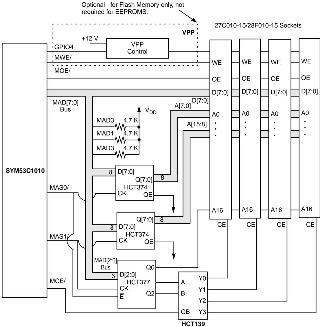
Note: MAD2 pulled low internally. MAD bus sense logic enabled for 512 Kbytes of slow memory (150 ns devices, additional time required for HCT139 @ 33 MHz). The HCT374s may be replaced with HCT377s.
