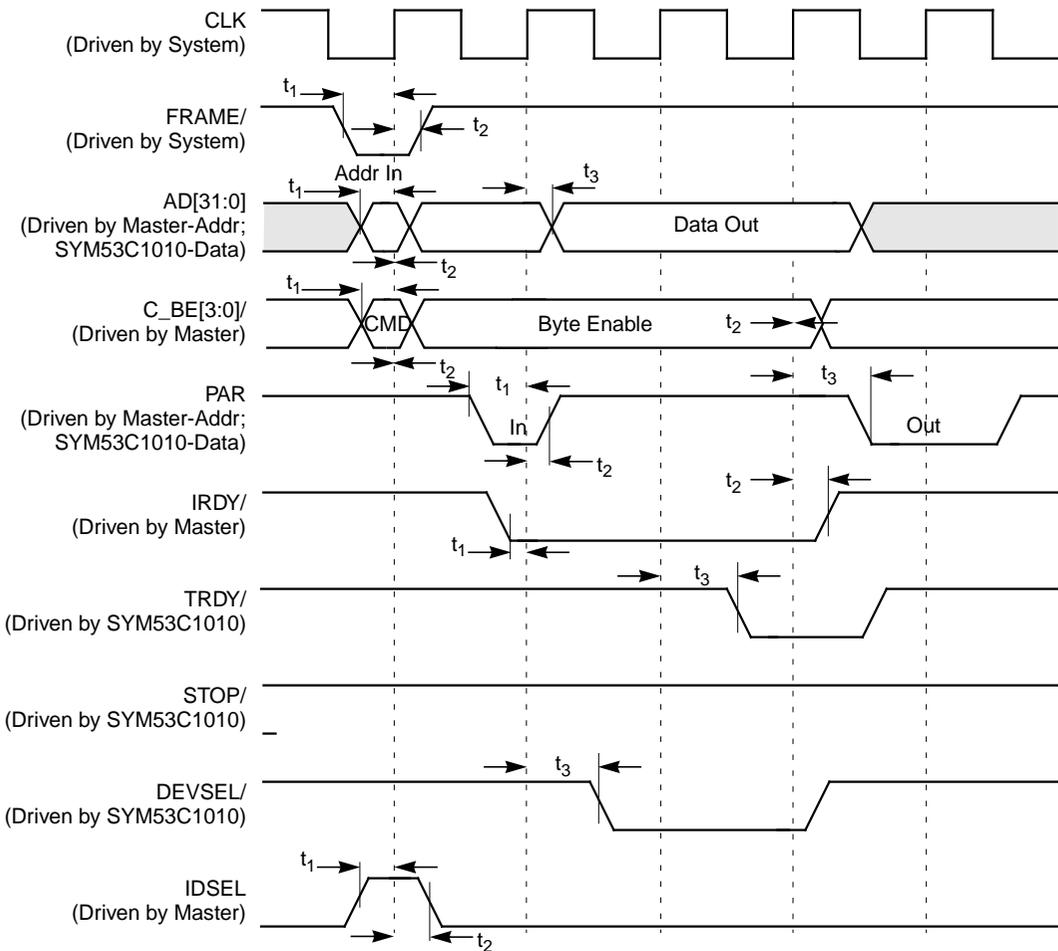
**Table 6.18 PCI Configuration Register Write**
