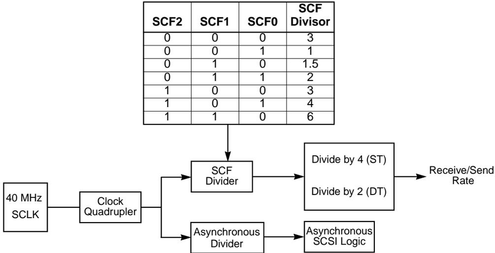
$$\text{Received Rate (DT)} = \frac{\text{Input Clock Rate}}{(\text{SCF Divisor} \times 2)} \quad (\text{megatransfers/s})$$
