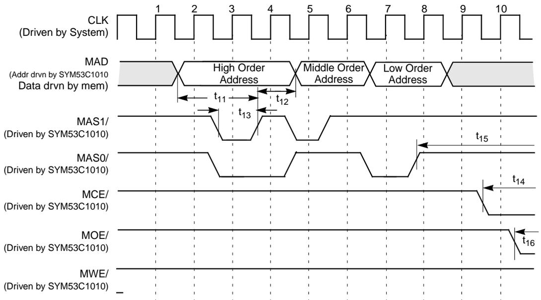
**Figure 6.31 Slow Memory ( $\geq 128$  Kbytes) Read Cycle (Cont.)**
