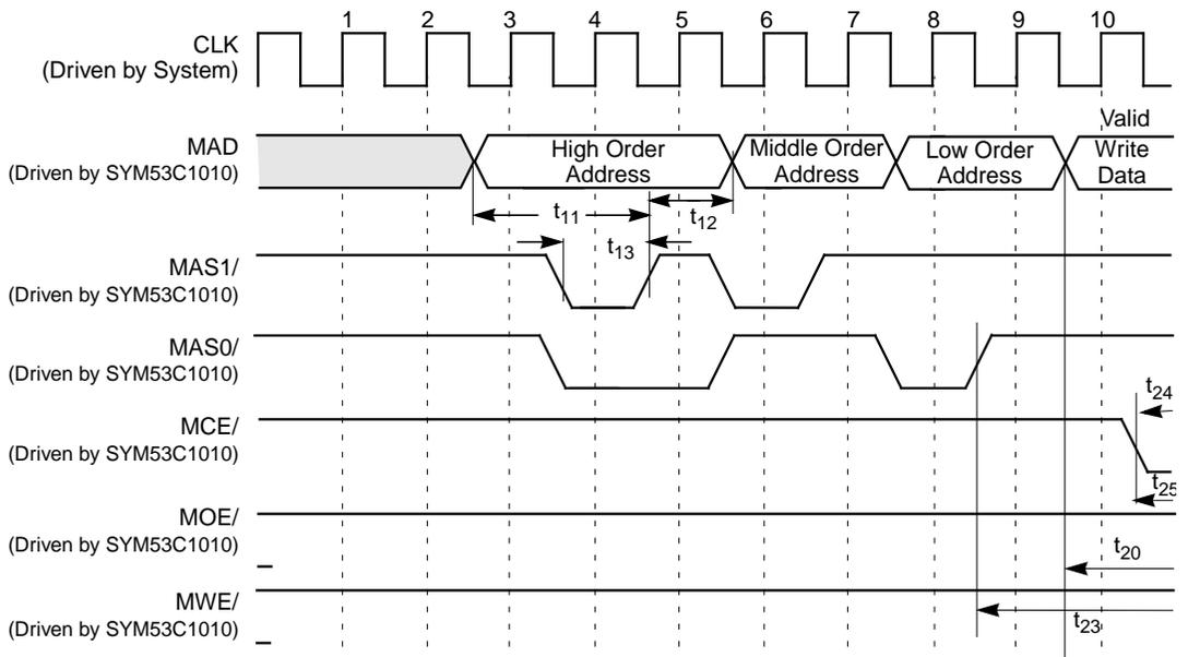
**Figure 6.32 Slow Memory ( $\geq 128$  Kbytes) Write Cycle (Cont.)**
