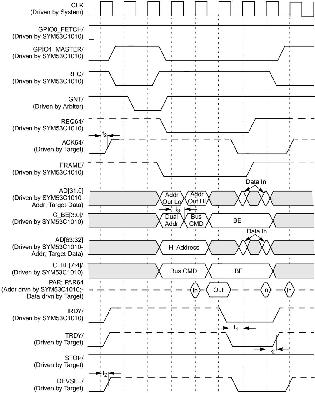
**Table 6.29 Burst Write, 32-Bit Address and Data**
