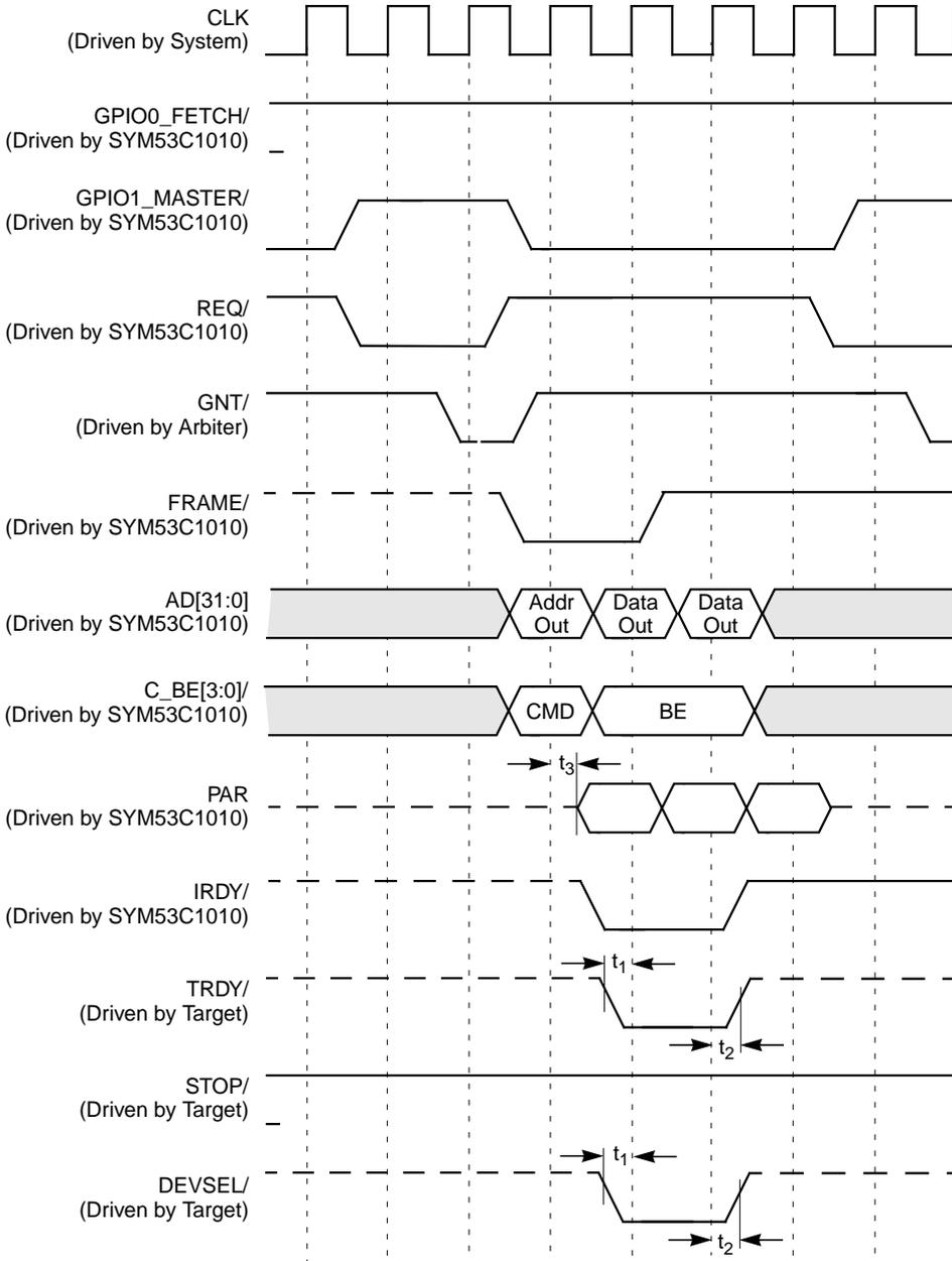
**Table 6.30 Burst Write, 64-Bit Address and Data**
