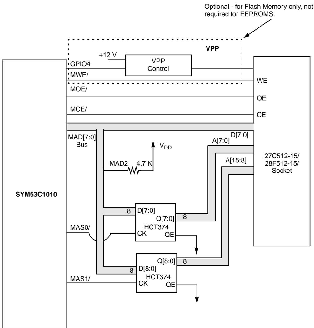
Note: MAD 3, 1, 0 pulled low internally. MAD bus sense logic enabled for 64 Kbyte of fast memory (150 ns devices @ 33 MHz).
