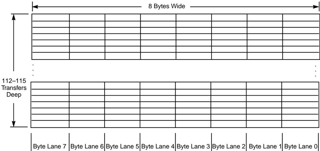
The SYM53C1010 supports 64-bit memory and automatically supports misaligned DMA transfers. The FIFO allows the SYM53C1010 to support 4, 8, 16, 32, 64, or 128 Dword bursts across the PCI bus interface.
