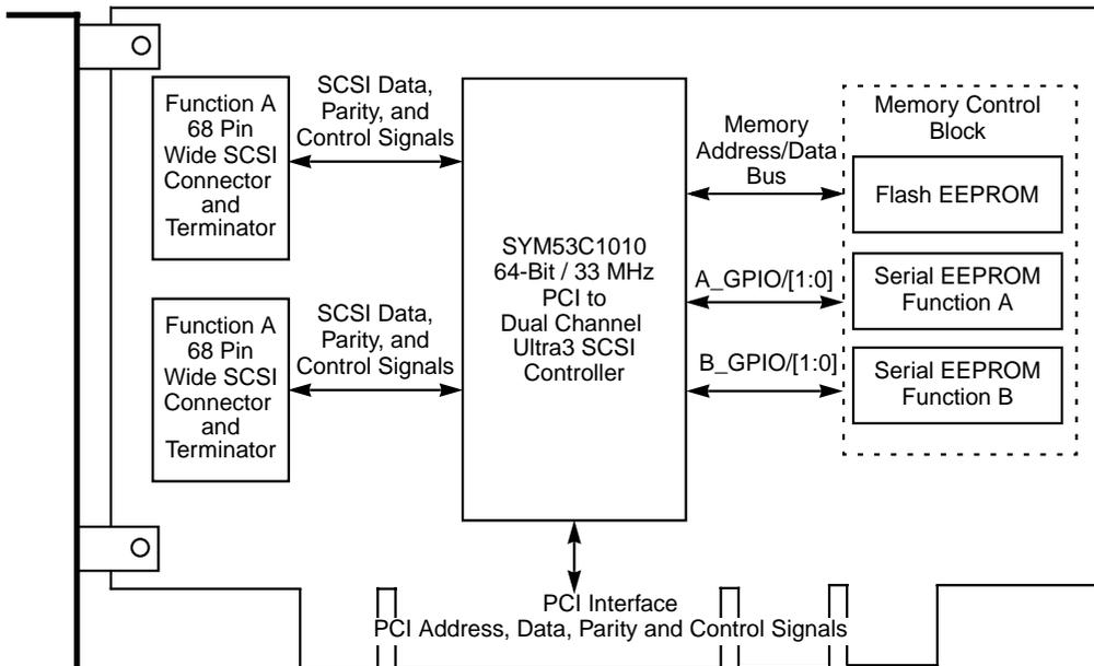
LVD Link™ technology is the LSI Logic implementation of Low Voltage Differential (LVD). LVD Link transceivers allow the SYM53C1010 to perform either Single-Ended (SE) or LVD transfers. The SYM53C1010 integrates two high-performance SCSI cores, a 64-bit/33 MHz PCI bus master DMA core, and the LSI Logic SCSI SCRIPTS™ processor to
