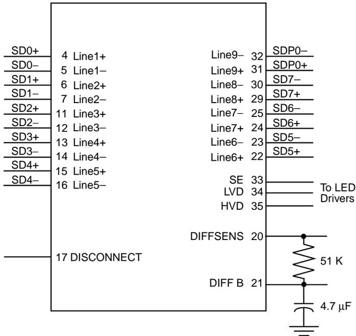
DIFFSENS connects to the SCSI bus DIFFSENS line to detect what type of devices (SE, LVD, or HVD) are connected to the SCSI bus. DISCONNECT shuts down the terminator when it is not at the end of the bus. The disconnect pin low enables the terminator.
