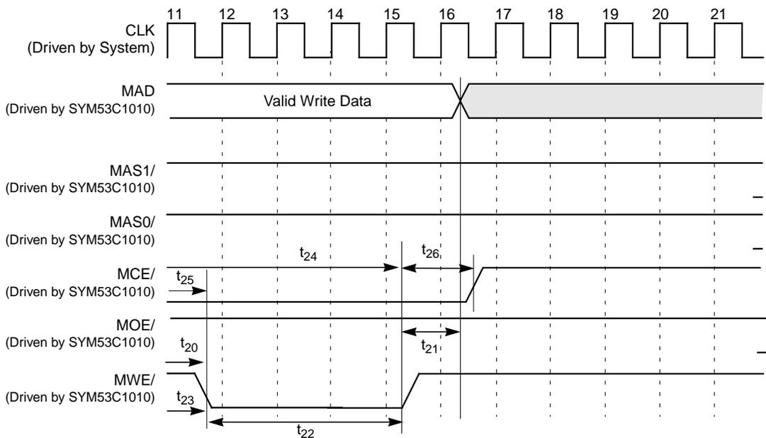
**Figure 6.29 Normal/Fast Memory ( $\geq 128$  Kbytes) Multiple Byte Access Read Cycle**
