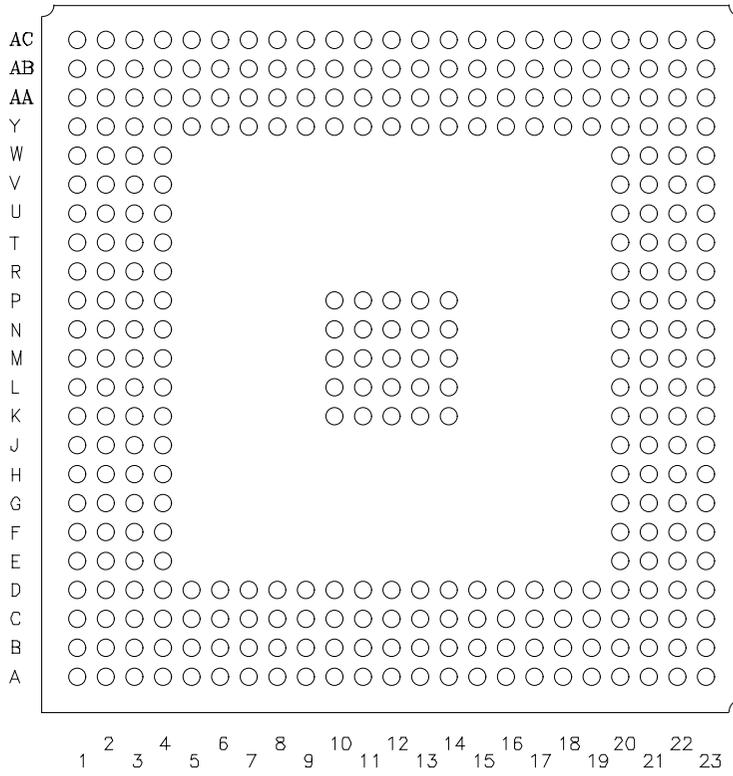
Figure 6.42 SYM53C1010-33 329 BGA Mechanical Drawing
