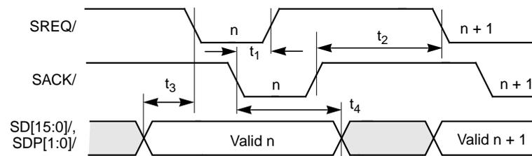
**Table 6.42 Target Asynchronous Receive**
