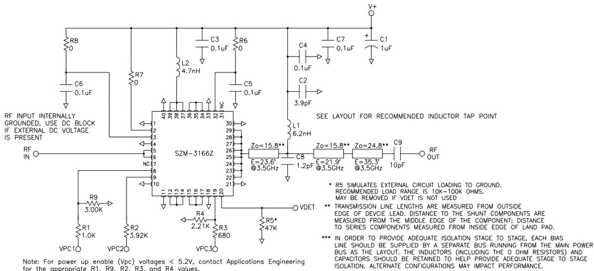
**3.3-3.6 GHz Evaluation Board Layout For Vcc = Vpc = 5.2V**
