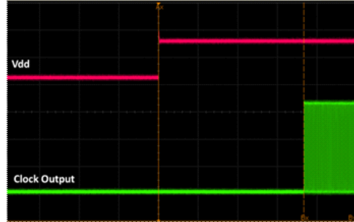
Figure 14. Startup Waveform vs. Vdd
