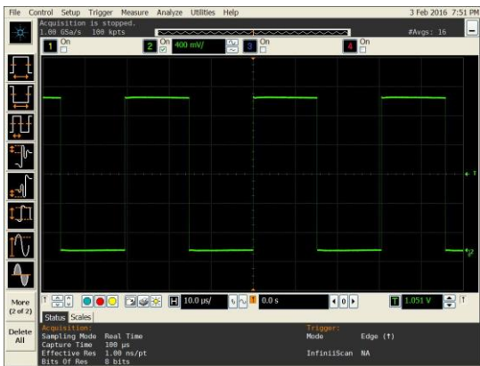
Figure 7. LVC MOS Output Sing
