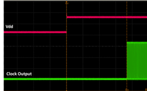
Figure 16. Startup Waveform vs. Vdd
