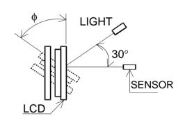
CONTRAST RATIO K VS VIEWING ANGLE  $\phi$  NOTE 4. DEFINITION OF OPTICAL RESPONSE
