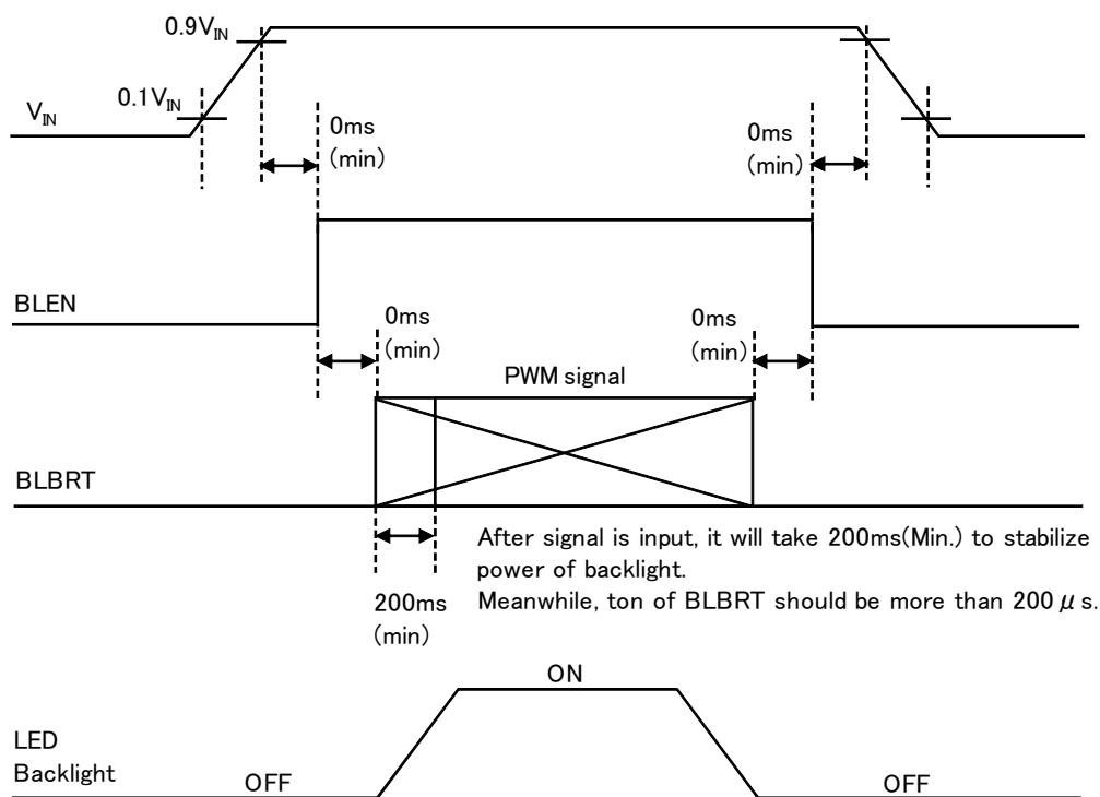
2)  $V_{IN} = 12V$ , Temp. =  $25^{\circ}\text{C}$ , DPWM = 100%
