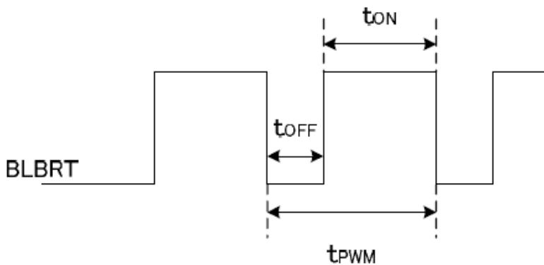
$t_{ON}, t_{OFF} \geq 50 \mu\text{s}$ .
