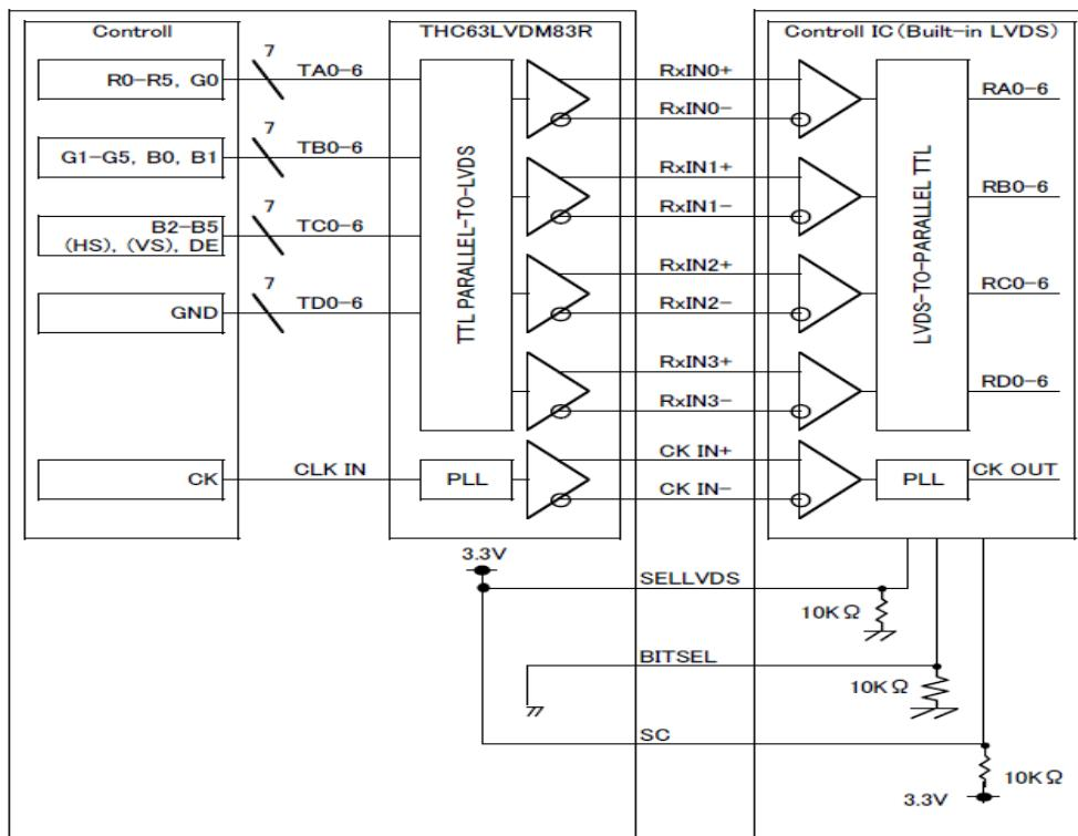
※SELLVDS signal line has  $10\text{ k}\Omega$  pulldown resister.
