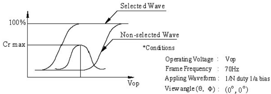
$$\text{Contrast ratio (Cr)} = \frac{\text{Brightness of selected dots}}{\text{Brightness of non-selected dots}}$$
