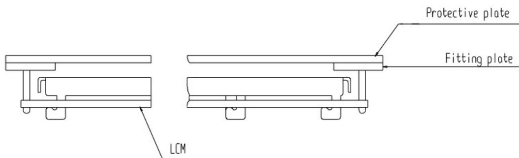
(2) When assembling the LCM into other equipment, the spacer to the bit between the LCM and the fitting plate should have enough height to avoid causing stress to the module surface, refer to the individual specifications for measurements. The measurement tolerance should be  $\pm 0.1\text{mm}$ .
