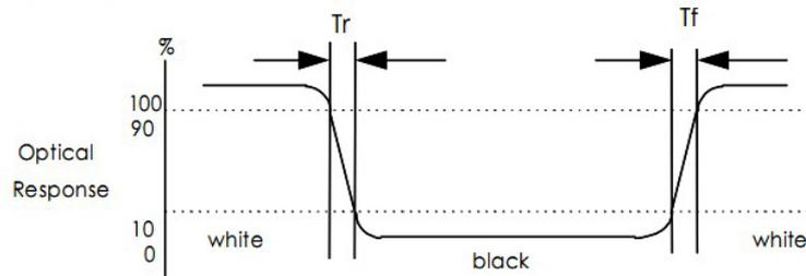
The values specified are at an approximate distance 500 mm from the LCD surface at a viewing angle of  $\theta$  and  $\phi$  equal to  $0^\circ$ . Measurement condition : Refer to next pages ( B - light source , Halogen Lamp, with polarizer )
