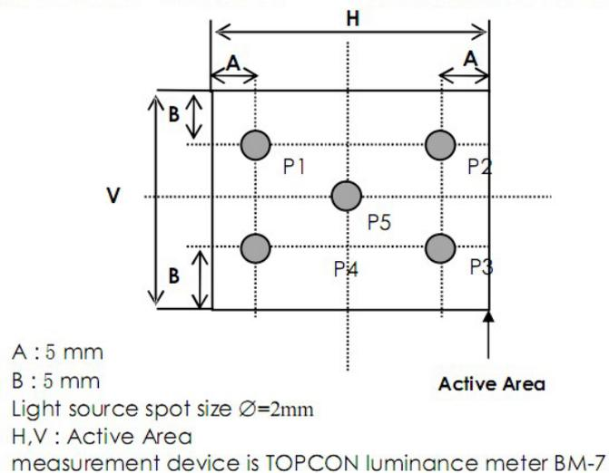
**FIG. 5 The definition of viewing angle**
