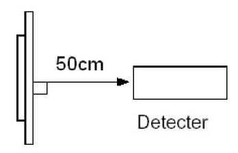
Note 2: The luminance uniformity is calculated by using following formula.  $\triangle Bp = Bp (Min.) / Bp (Max.) \times 100 (\%)$
