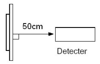
Note 2: The luminance uniformity is calculated by using following formula. ⊿Bp = Bp (Min.) / Bp (Max.)×100 (%)
