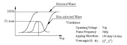
Contrast ratio (Cr) = Brightness of selected dotsBrightness of non-selected dots
