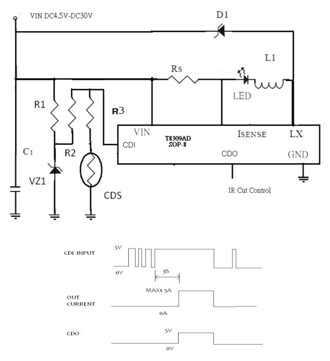
\* note : When outputs the big current, the noise are big, this and the system environment and PCB layout have the influential, may defer to the actual need to increase the capacitor filtration noise.
