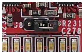
Figure 7-4 VCC_ADJ SEL Jumper
