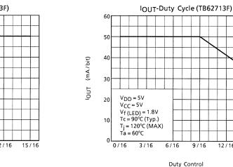
IOUT-Duty Cycle (TB62713F) 60 50 40 (mA / bit) 30 lout  $V_{DD} = 5V$   $V_{CC} = 5V$   $V_{f}$  (LED) = 1.8V  $T_{c} = 80^{\circ}C$  (Typ.)  $T_{j} = 120^{\circ}C$  (MAX)  $T_{a} = 40^{\circ}C$ 20 10 ol 0/16 3/16 6/16 12/16 9/16 Duty Control
