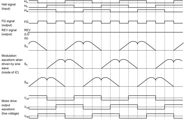
\* The waveform of actual operation is the PWM
