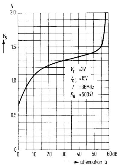
**Tuner control current versus attenuation**
