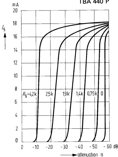
**Tuner control current versus attenuation**
