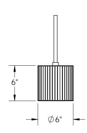
Specification: Construction: Extruded aluminum fluted cylindrical housing. Electrical: CSA/UL approved electronic power supply. Finish: 3 stage powder painted.
