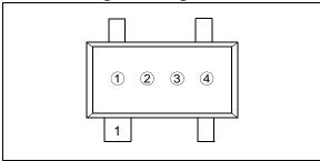
① & ② = part number code + threshold voltage (two-digit code)
