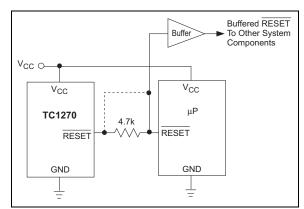
FIGURE 4-3: Interfacing to Bidirectional Reset I/O.
