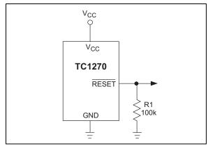
**FIGURE 4-2:** Ensuring  $\overline{RESET}$  Valid to  $V_{CC} = 0V$ .
