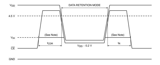
Note: When  $\overline{CE}$  is operating at the V<sub>IH</sub> level (2.2V), the standby current is given by I<sub>DDS1</sub> during the transition of V<sub>DD</sub> from 4.5 to 2.4V.
